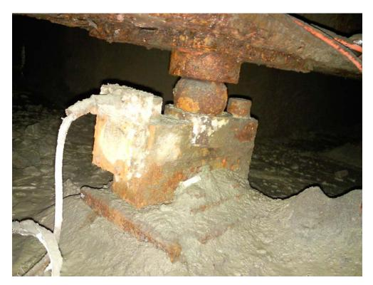
• Stainless Steel materialized load cells to prevent rust and corrosions
